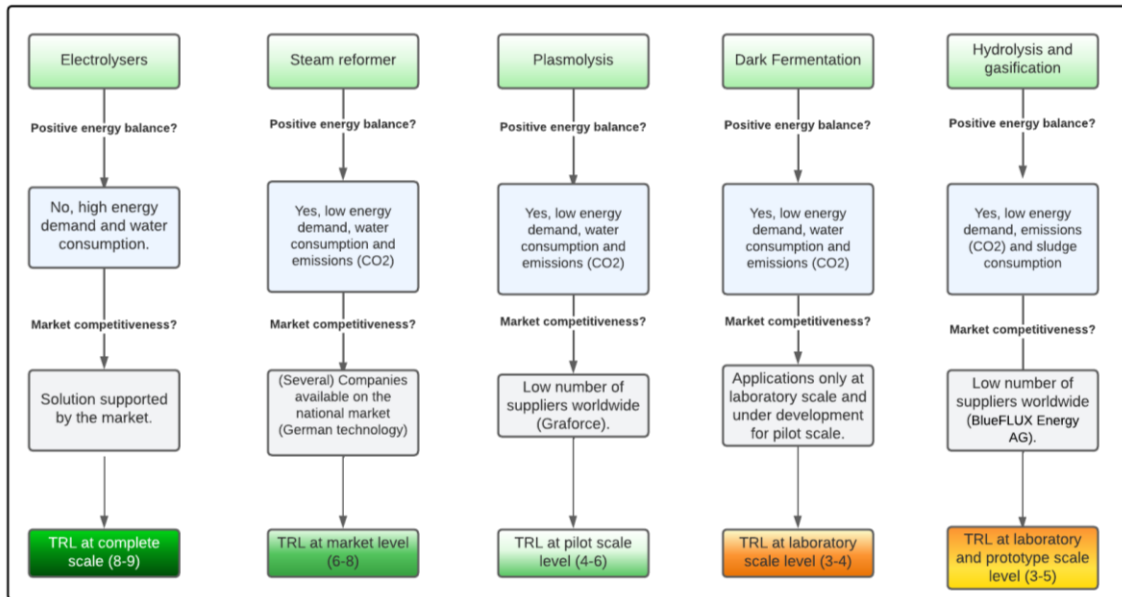
Figure 3 - Comparison matrix of technological routes for hydrogen production Source: Prepared by the authors, 2023.
